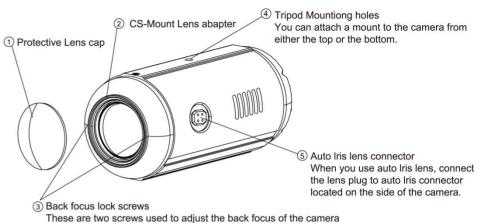
which is normally set on factory default. These must be loosened (using an L-wrench) before the camera can be focused. after readjsting, lock the screws into place.
