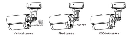
Fix the bracket in camera setting place, and then set the camera in it.
