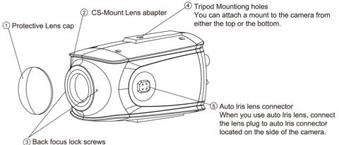
These are two screws used to adjust the back focus of the camera which is normally set on factory default. These must be loosened (using an L-wrench) before the camera can be focused. after readjsting, lock the screws into place.
